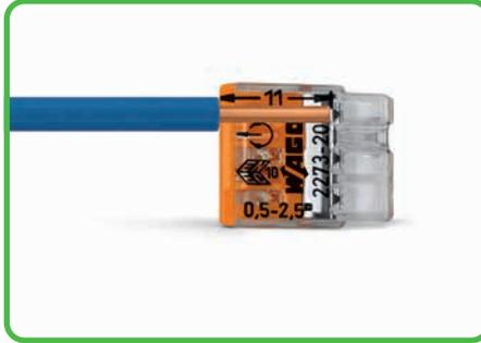
Strip solid conductor to 11 mm (see marking). Conductors are correctly stripped if the clear port shows no bare conductor on the unprinted connector side. Picture shows center conductor with exceeded strip length.
